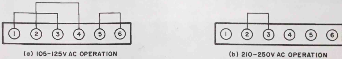
Figure 1.7. TB1 Jumper Positions
