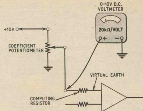
Fig. 4.3. Voltmeter method of determining coefficient potentiometer settings
