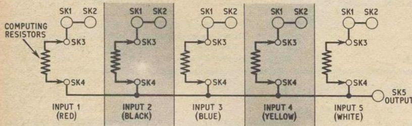
Fig. 2.8. Circuit diagram of Summer 1, 2, and 3
