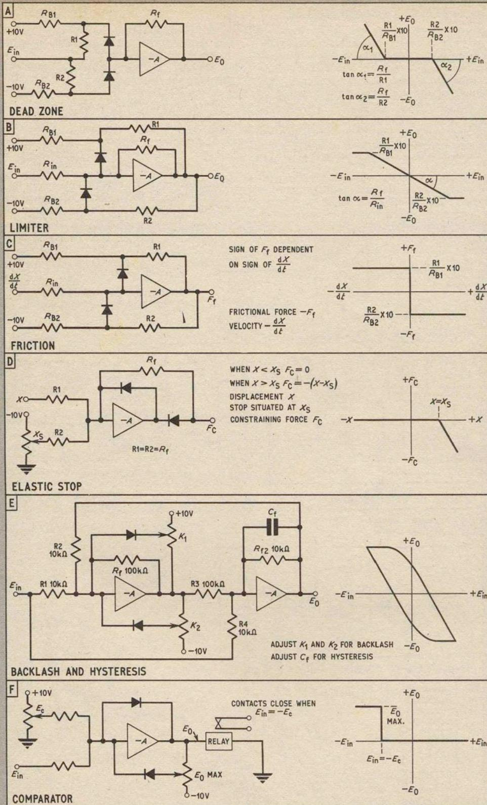
Fig. 10.2. Special circuits for simulating mechanical phenomena
