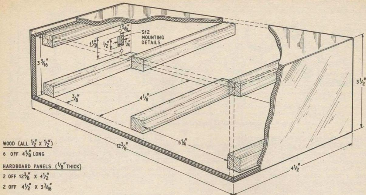
Fig. 9.4. Construction of the box for UNIT "D"
