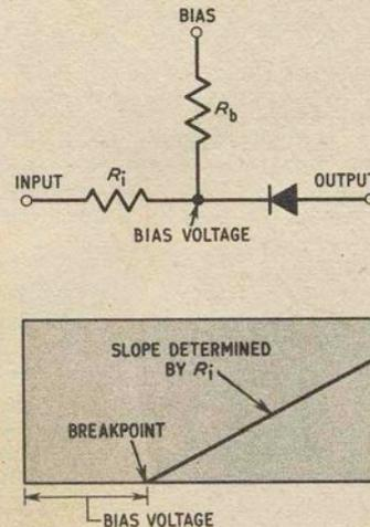
Fig. 1.4a (left). Illustrating how a mathematical function can be constructed from a series of straight line tangents
