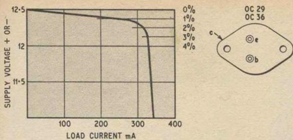
Fig. 3.2. Performance curve of stabilised power supply
