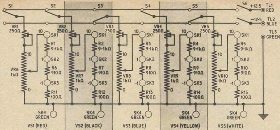
Fig. 2.6. Circuit diagram of Voltage Source section
