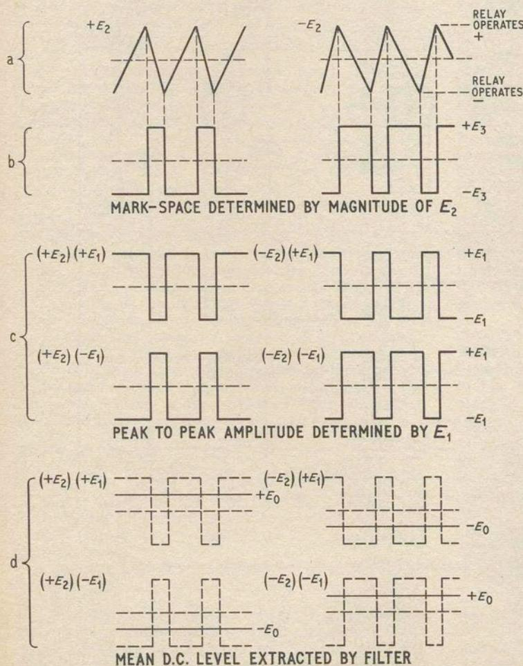
Fig. 9.1. Time division multiplier with associated waveforms
