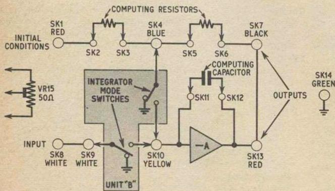
Fig. 2.9. Circuit diagram of Operational Amplifier 1, 2, and 3
