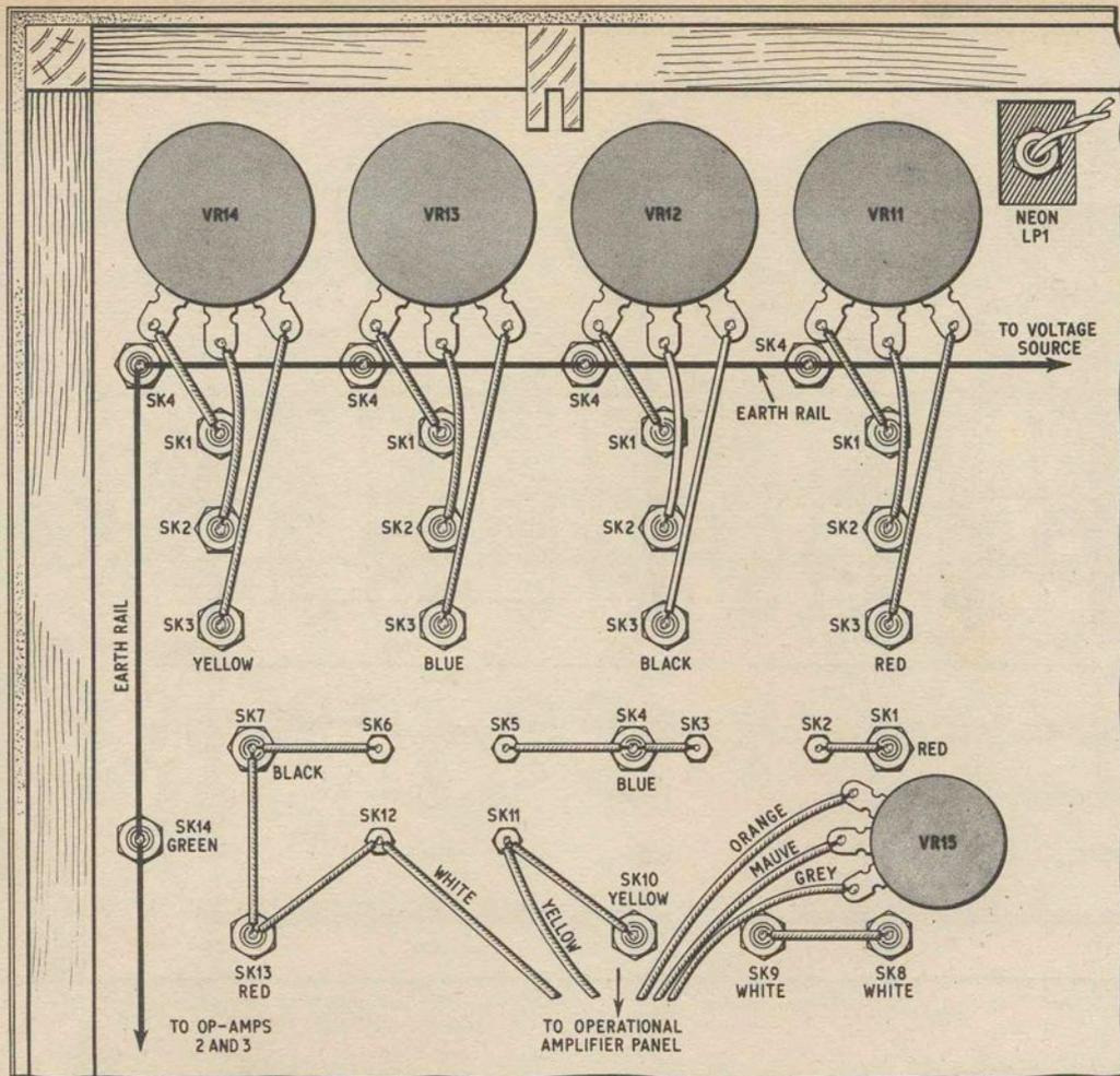
Fig. 2.4. Right-hand portion of front panel viewed from rear, showing components and wiring. Operational Amplifiers 2 and 3 are wired exactly as "Operational Amplifier 1" shown here
