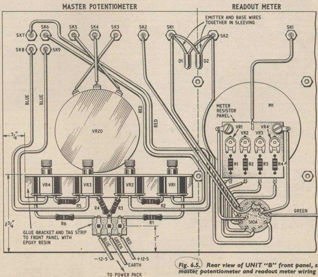
Fig. 6.5. Rear view of UNIT "B" front panel, showing master potentiometer and readout meter wiring
