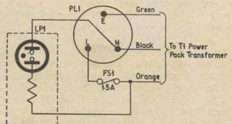
Fig. 2.10. Circuit diagram of mains supply
