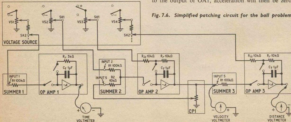
Fig. 7.6. Simplified patching circuit for the ball problem
