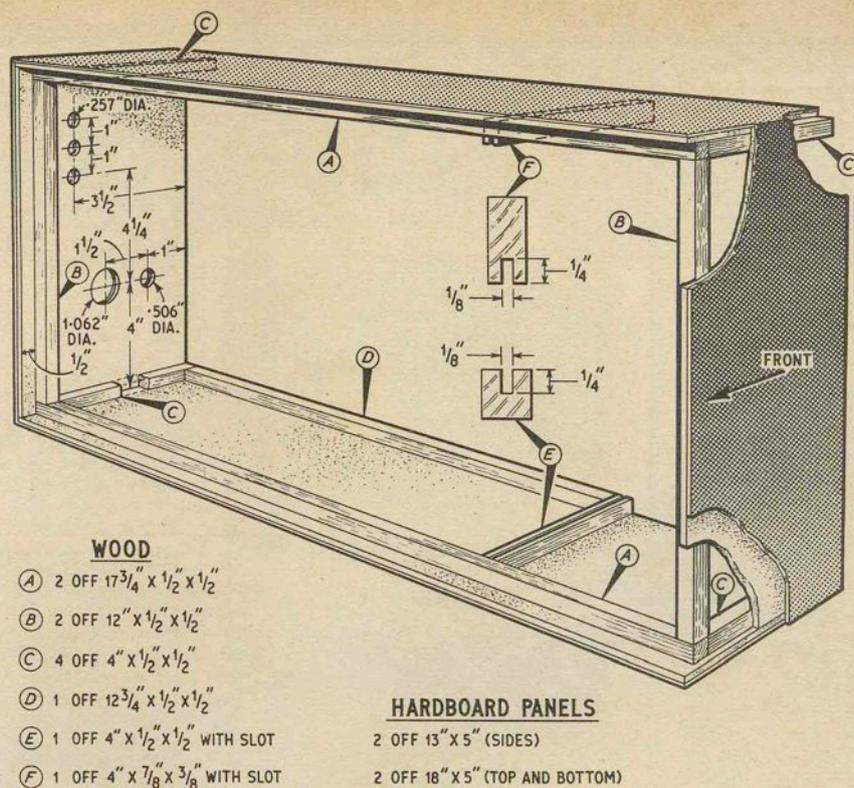
Fig. 2.12. Constructional details of UNIT "A" Box
