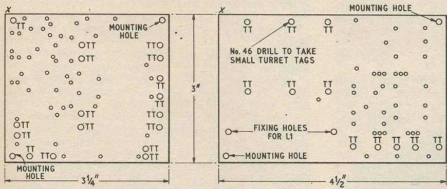
Fig. 9.6 (far left). Top and underside views of bistable relay panel
