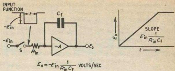
Fig. 5.1. The operational amplifier as an integrator
