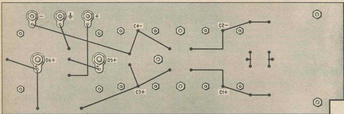
Fig. 3.5 Underside wiring of power supply panel
