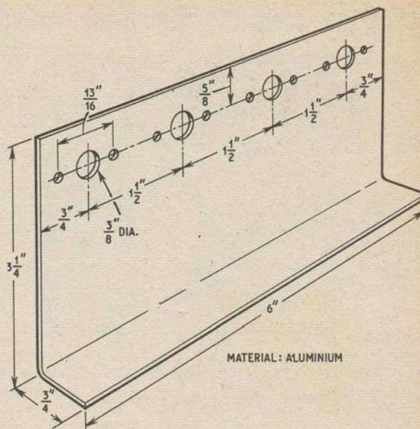
Fig. 6.6. Mounting bracket for pre-set potentiometers
