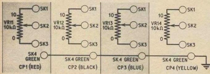
Fig. 2.7. Circuit diagram of Coefficient Potentiometers section
