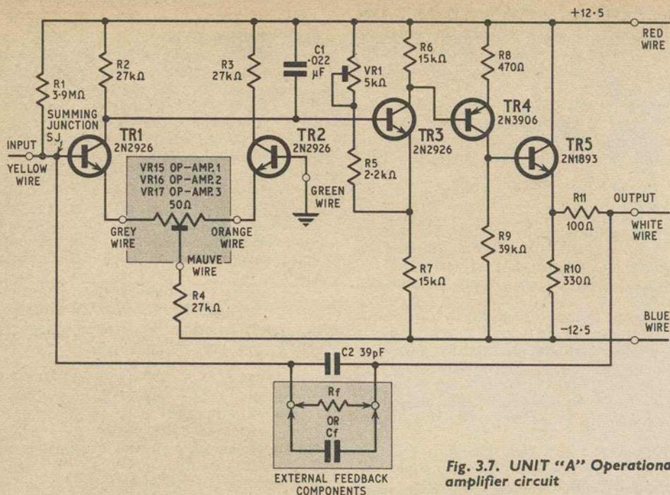
Fig. 3.7. UNIT "A" Operational amplifier circuit
