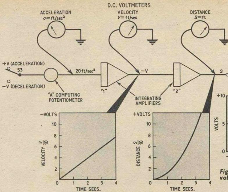
Fig. 1.3a (left). The use of integrators is illustrated in this diagram. In this example the rate of acceleration, velocity, and distance covered by a motor car are computed and can be read off the potentiometer dial and meter scales
