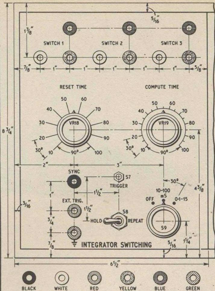
Fig. 6.1. UNIT "B" front panel, integrator switching section
