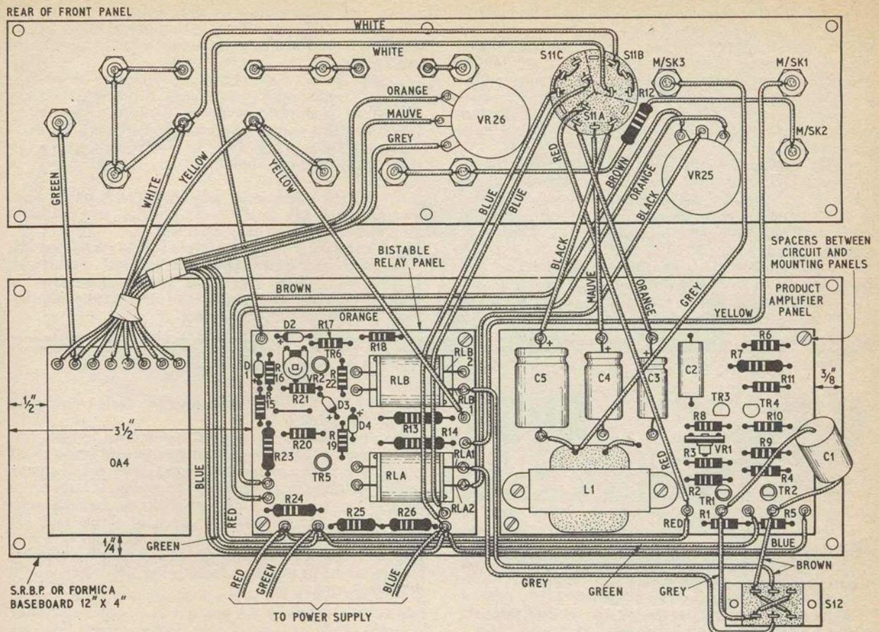
Fig. 9.5. Internal layout and wiring of UNIT "D" multiplier
