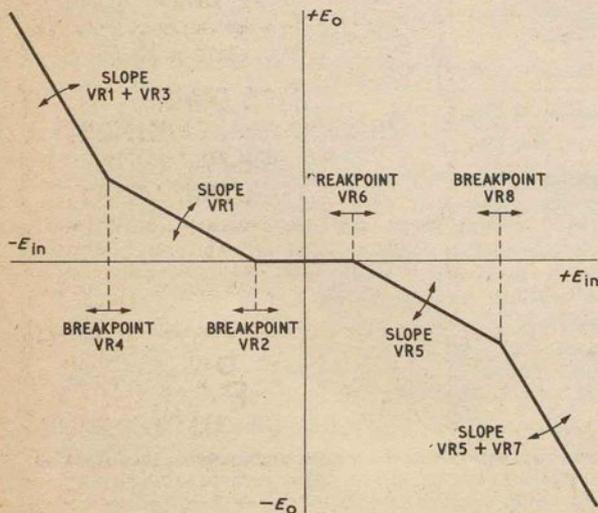
Fig. 7.8b. Adjustable characteristic of simple function generator
