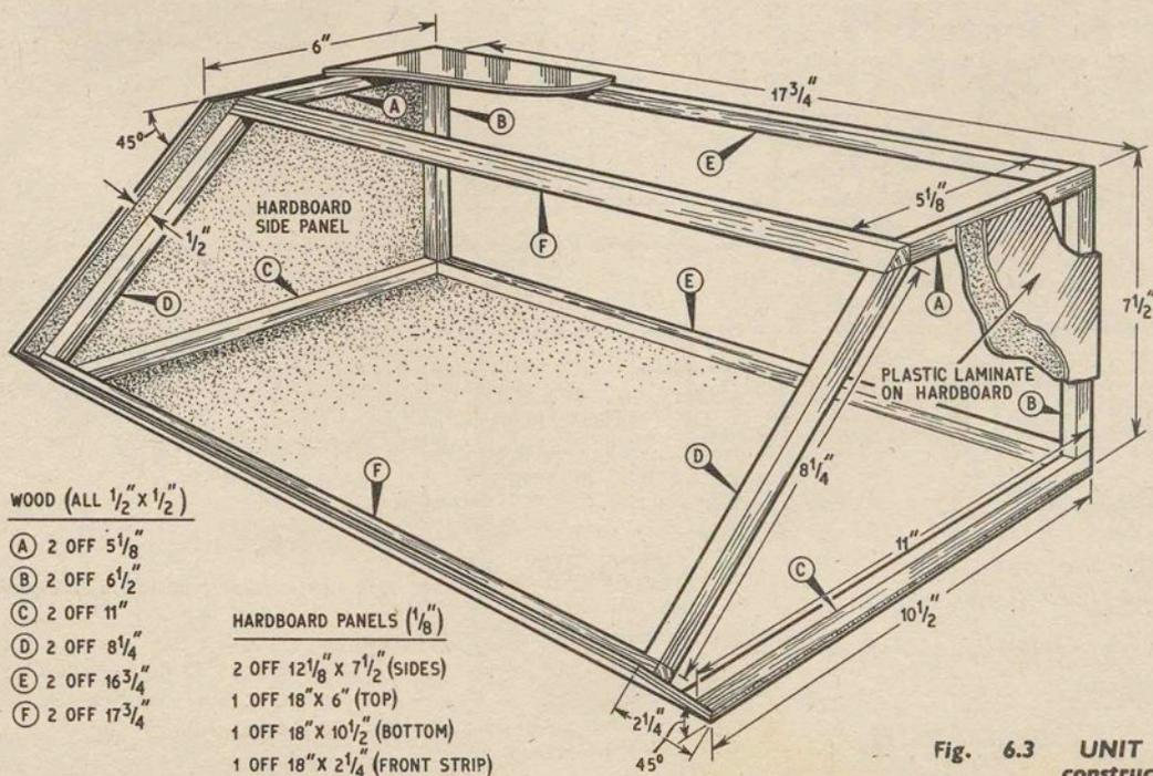
Fig. 6.3. UNIT "B" box constructional details
