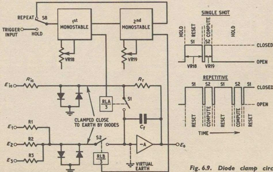
Fig. 6.9. Diode clamp circuit, showing principle of operation
