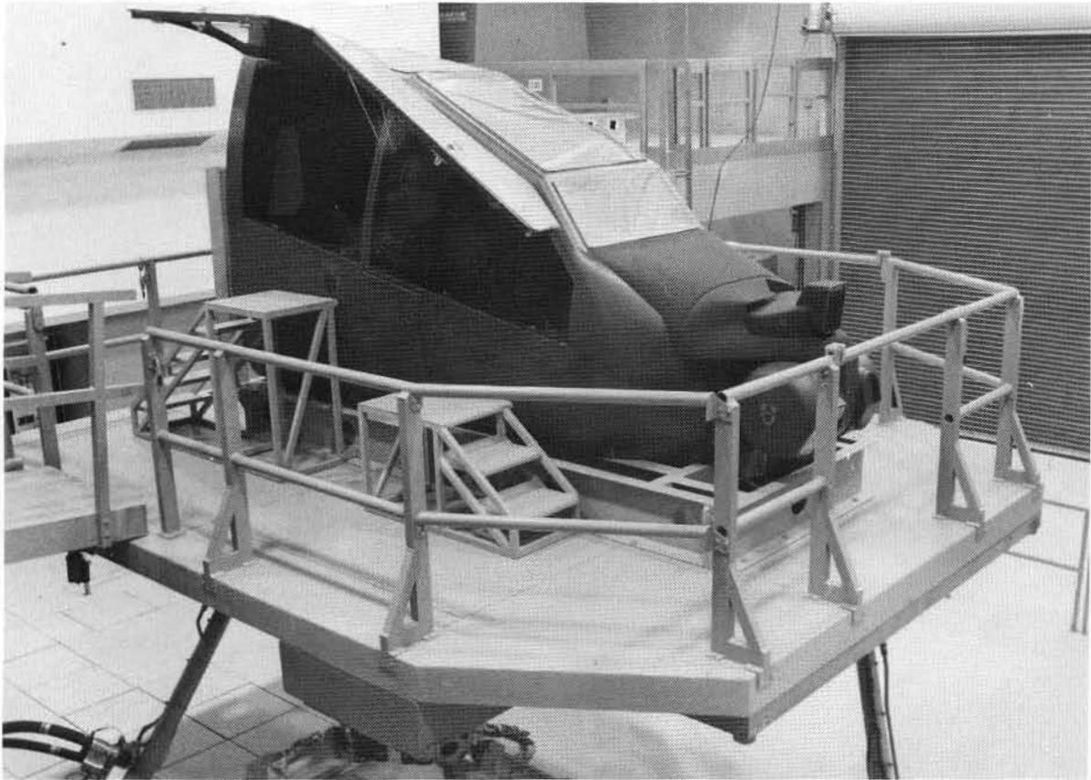
Figure 7. 6 DOF Motion Base and Cockpit
