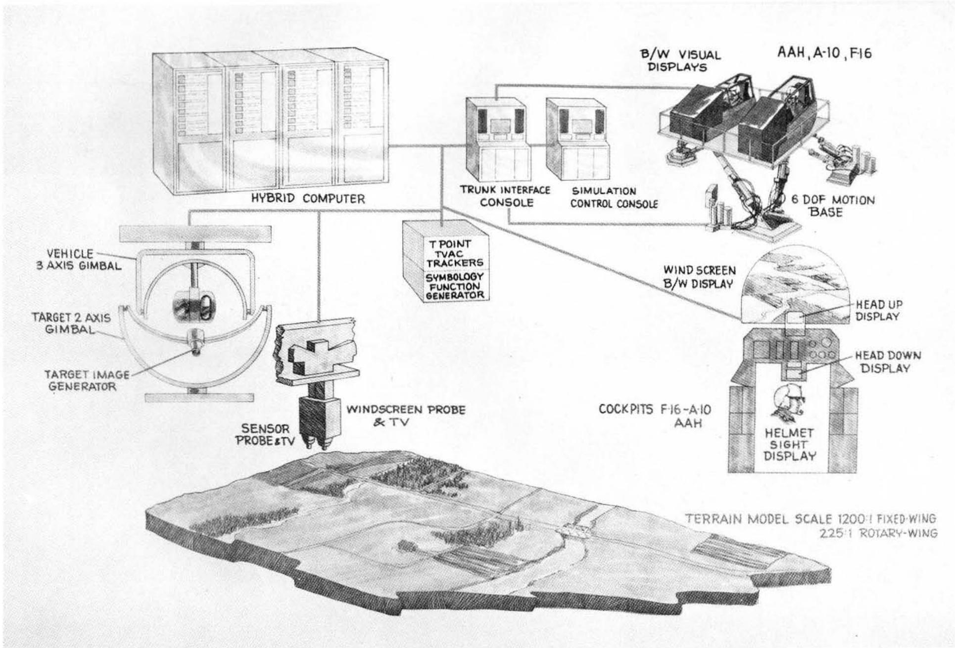
Figure 2. Simulation Elements
